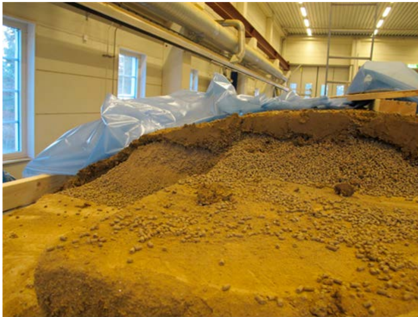
Figure 5-15. Photo showing a cross section (close to the installed geotextile) of the pellet filling at the top of the tunnel in Test 5. It is obvious that the inflowing water has followed the geotextile up over the crown and down on the other side of the tunnel (inflow side to the left in the photo). However, as shown in the photo, there is a remaining dry layer of pellets close to the block stack.
