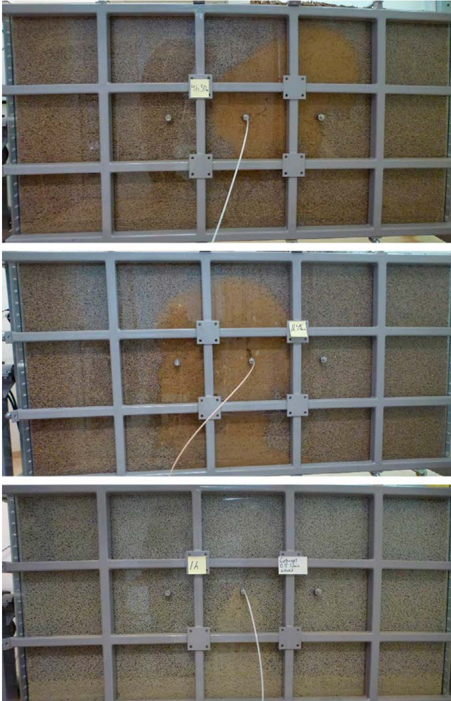
Figure 5-11. Upper: Photo showing an example of “Symmetric/Upwards” wetting. Middle: Photo showing an example of “Symmetric” wetting. Lower: Photo showing an example of “Downward” wetting.
