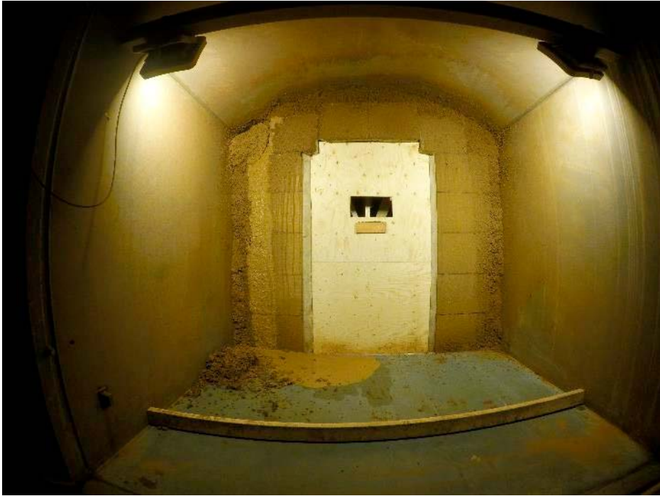
Figure 5-6. Photo showing the first water breakthrough in Test 4.
