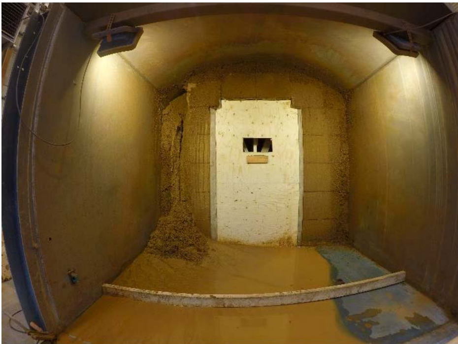
Figure 5-7. Photo showing the backfill front of Test 4 at time for termination.
