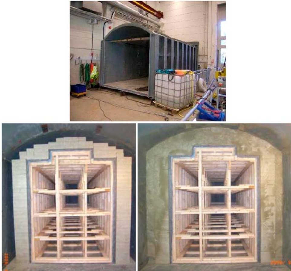
Figure 5-23. Photographic images of SKB 1/2-scale steel tunnel mock-up (upper photo), undertaken at Äspö HRL (Dixon et al. 2008b, 2011). The block assembly prior to installation of dry pellet fill (lower left photo) and wetted pellet wall used in later tests (lower right photo) (Dixon et al. 2011).
