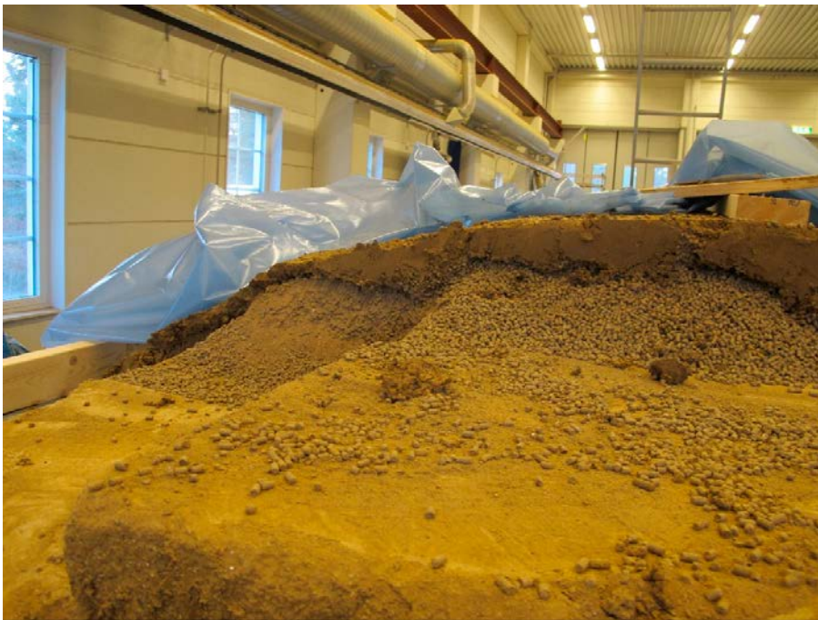
Figure 5-10. Photo showing a cross section of the pellet filling at the top of the tunnel in Test 5. It is obvious that the inflowing water has followed the geotextile up over the top and down on the other side of the tunnel (inflow side to the left in the photo).
